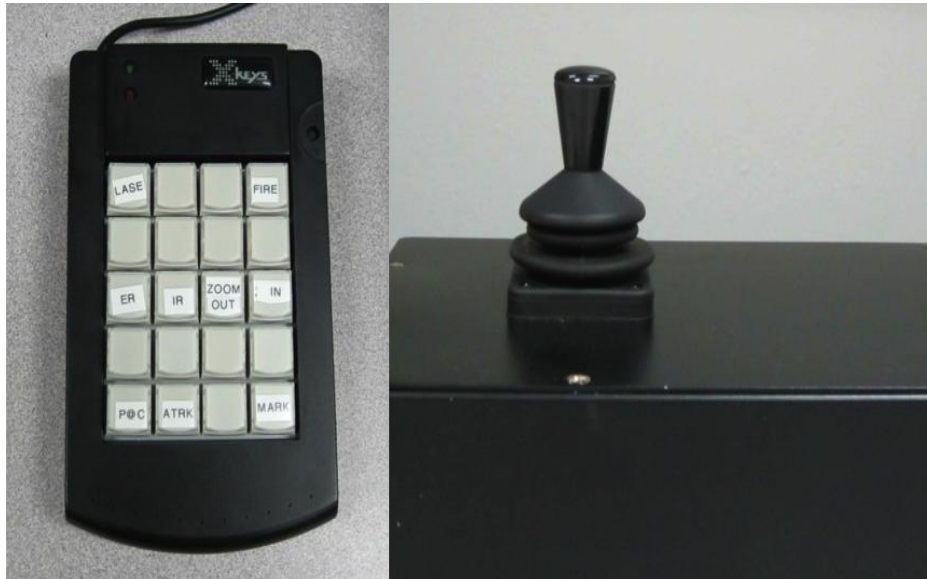
Figure 6 – Universal Ground Control Stations Joystick and P.I. Engineering X-keys MWII input devices
